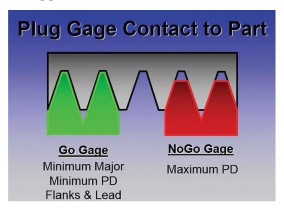
With the same principles as thread plugs, thread ring gages also work in the same fashion. The only difference here is that a Go thread ring is measuring the maximum minor diameter instead of the minimum major diameter. The major diameter is not measured with either the Go or No-Go ring. That is measured with a separate gage such as an OD micrometer. Like the No-Go thread plug, the No-Go thread ring is only verifying that the pitch diameter is within allowable limits.
