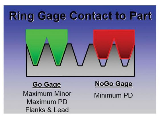
For this reason, it is very important to check the hole with the No-Go gage and the Go gage every time an adjustment is made to cutter compensation. It should never be assumed that compensation be continually made until the Go thread gage is accepted, as this side of the gage is checking more features of the thread than the No-Go thread gage.
