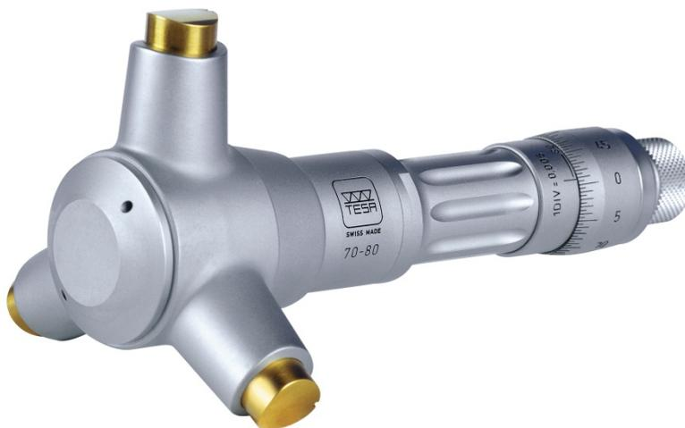
Internal micrometers from the TESA IMICRO range offer a market advantage. Their unique technology offers a precise and quick measurement of cylindrical bores. In fact, the drive of the measuring anvils via the spiral measuring cone allows linear control of the displacement of the instrument. In addition, the ratchet allows a constant measuring force.
