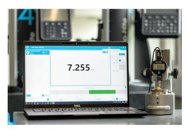
TESA DATA-VIEWER allows a quick and easy handling in order to export the results to a data processing program or to automatically create files in known formats such as \*.xls, \*.csv or \*.txt.
