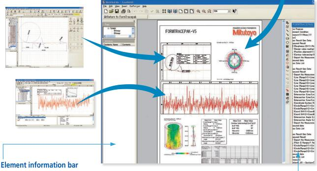
This bar displays the attribute values of the pasted items, allowing you to easily check the contents of the pasted measurement data files.
