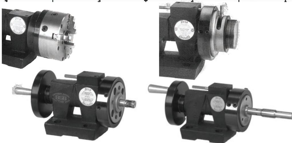
The GSG Zero spindle offers various methods of holding a part on the inside feature during rotation. The charts show the 4 major methods: Collet, push arbor, 3-4 Jaw Chuck, and internal off Lead Lock. These methods can be combined with various measurement methods and provide the user with a robust and repeatable way of inspecting ovality, run-out, diameter and true position of round parts.
