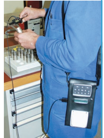
The above illustration shows the use of the Statistics Printer in the Transport Bag MSP 2t
