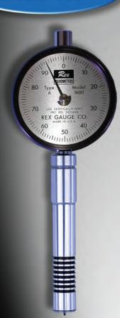
Conforms to ASTM D-2240
